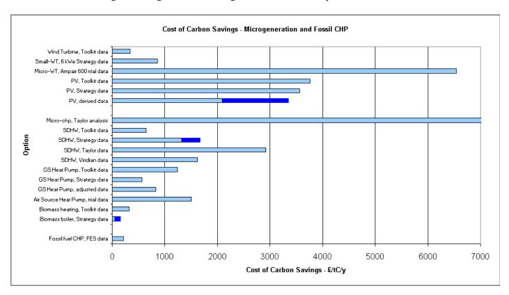
This shows that the lowest cost carbon savings are with biomass heating and fossil CHP. Due to scale effects on performance and specific cost, these measures are best implemented at large scale, and thus off-site. Hence they are applicable to the urban domestic residential sector, as well as the commercial and industrial sectors.
