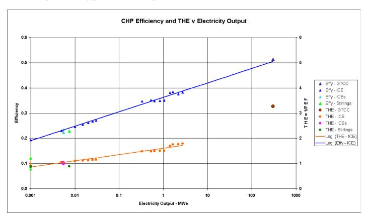
It shows - in blue - the Electricity Efficiency for Internal Combustion Engines (ICEs) ranging from 1 kWe to around 1 MWe, plus that for a Gas Turbine Combined Cycle plant of 300 MWe.
