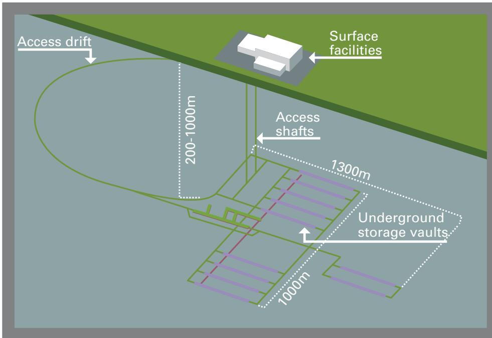
Figure 8.1: A generic design for ILW disposal concept: the waste would be immobilised in concrete and placed underground
