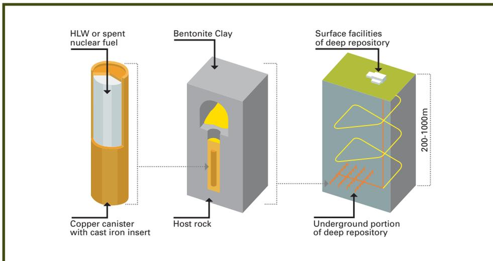
Figure 8.2 A generic design for high level waste and spent fuel disposal: the material would be encapsulated in copper canisters and then placed in deposition tunnels underground
